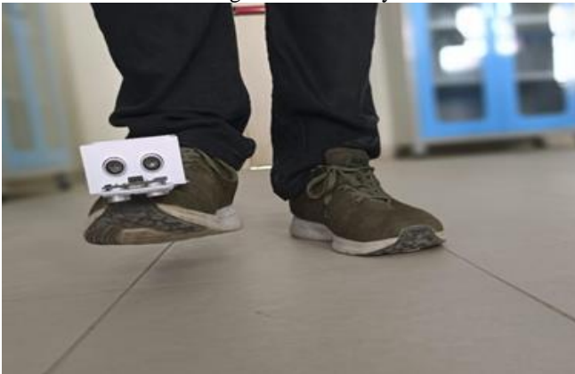
Fig. 5. Implementation of Smart Device on Shoes
